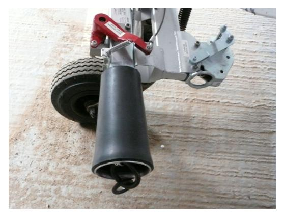
New aerotow rope attachment on the Pawnee (tail-wheel is turned sideways)
